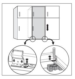
Align the appliance on both side using the adjustable feet.
